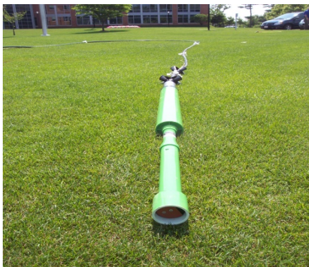
Submersible pump sand separator for sediment isolation and removal from pump intake (Hingham, MA)
