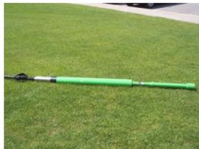
Submersible pump sand separator for sediment isolation and removal from pump intake (Stoughton, MA)
